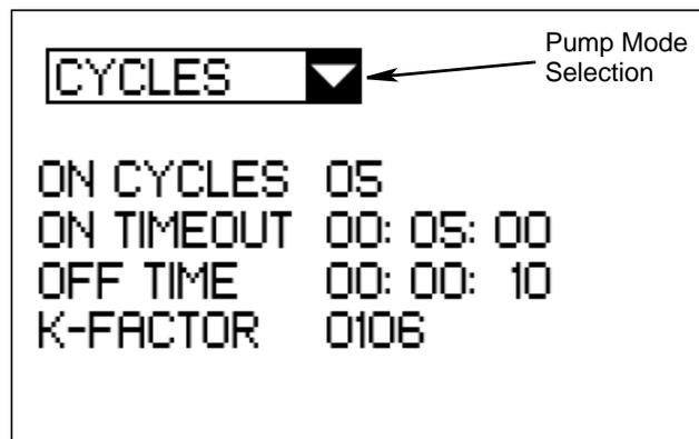
**FIG. 9: Pump Setup screen (Cycle mode)**
