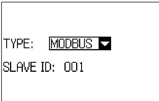
FIG. 22: Network Setup screen
