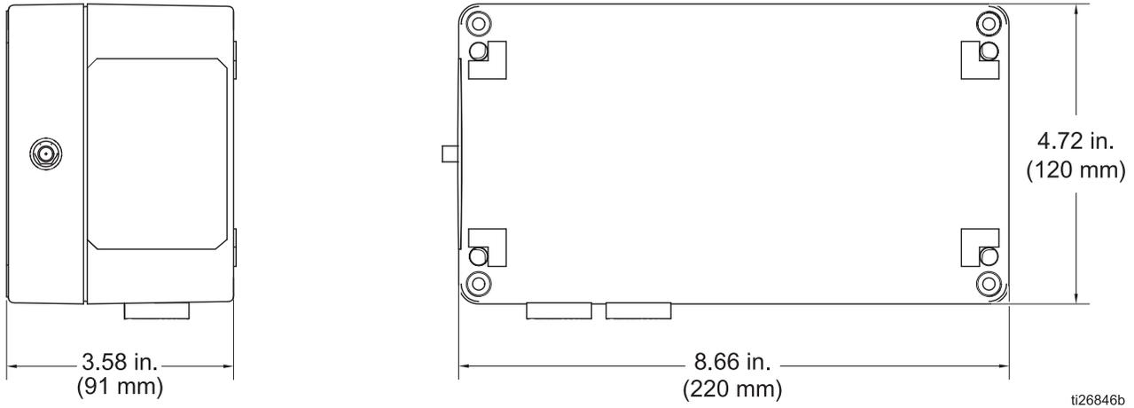
**FIG. 43: Harrier+ Dimensions and Mounting Hole Layout**
