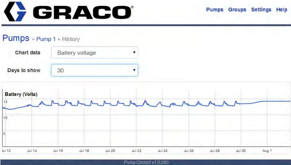
**FIG. 32: History Chart of Battery Voltage for 30 days**
