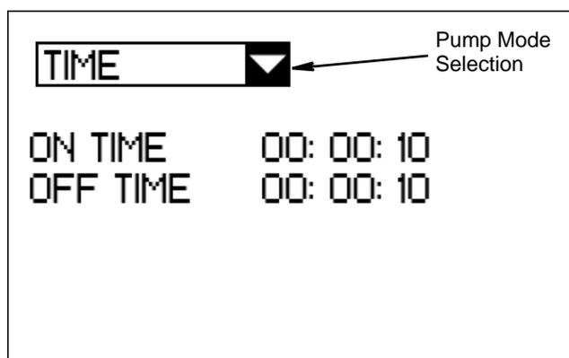
**FIG. 8: Pump Setup screen (Time mode)**
