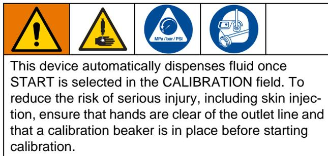
2. Only if pump calibration is needed, highlight CALIBRATION and press Enter.
