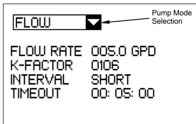
**Fig. 7: Pump Setup screen (Flow mode)**
